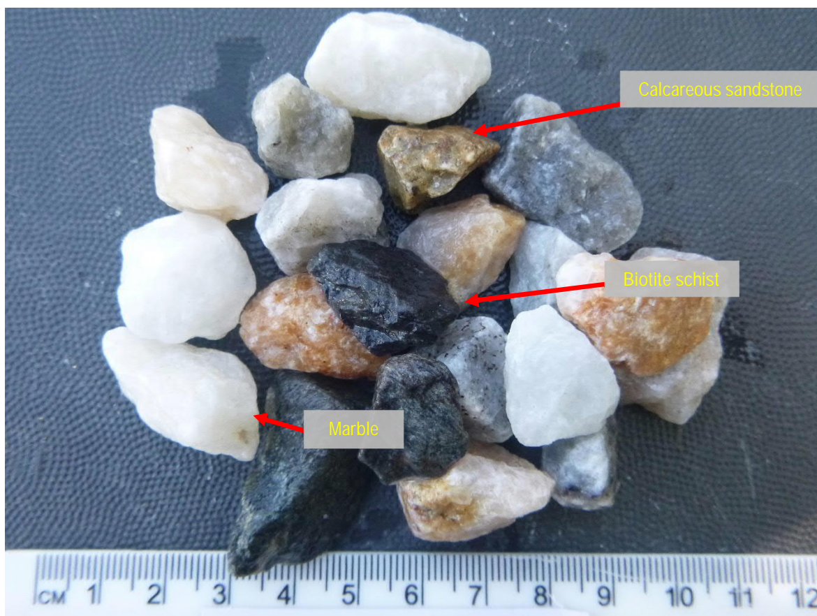
Plate 2: Photograph of the washed sample, shows the abundance of the different lithologies.
