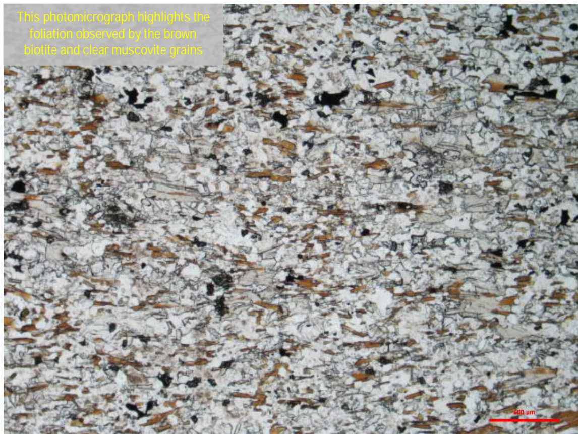
Plate 5: Microphotograph of the biotite schist lithology at 40x magnification utilising plane polarised light. Scale = 500µm x 40 magnification. F.O.V 5.2mm.
